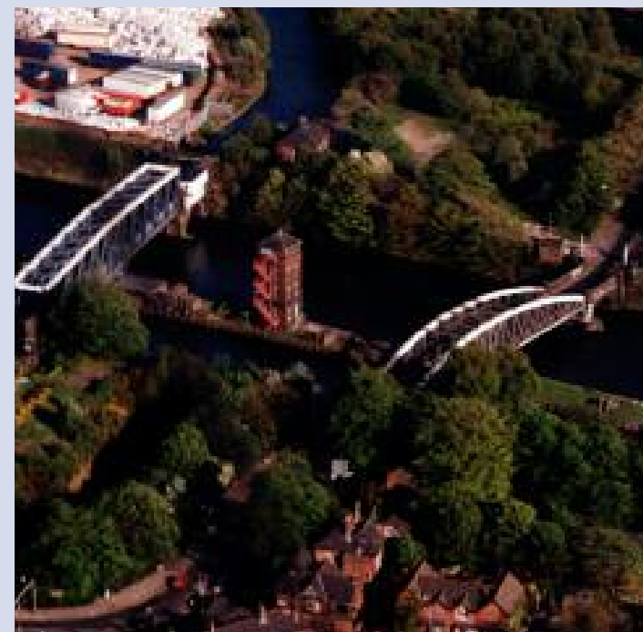
photo: Barton-on-Irwell showing (left) the swing-aqueduct carrying the Bridgewater Canal over the Manchester Ship Canal and (right) the Barton road bridge. photo by RuthAS
